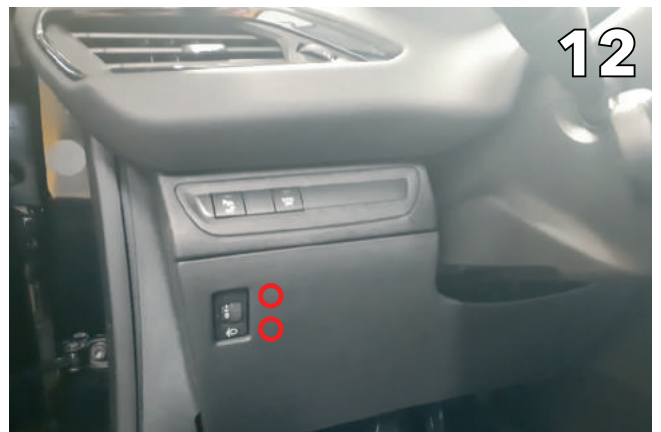
Proposed locations for traction control button and tire pressure reset button
