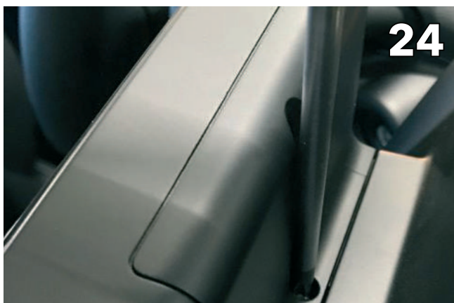
Slide the connector cover in the back of the screen and fix the screw (included with SPH-EVO62DAB-208)
