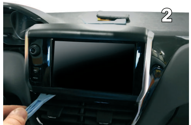
2 Remove front cover by lifting up as shown
