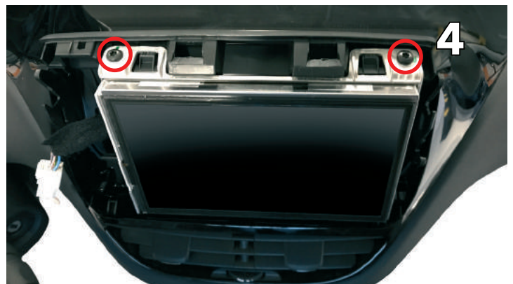
4 Remove two Torx screws on top
