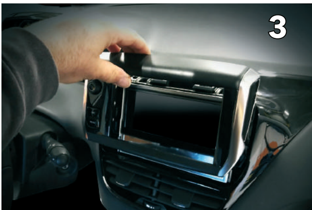
3 Pull upwards to remove and disconnect buttons
