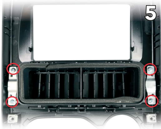
5 Re-install the vents (if you have a pre-facelift vehicle: use the two metal tabs to support the vents)
